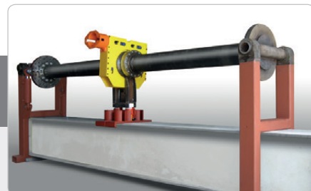
Vector Optima® full scale pressure and bending test
